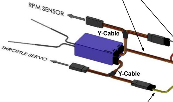
Plug the glow-plug cable into the bottom port and add the throttle pickup wire (SKU: AAVXG0204)
