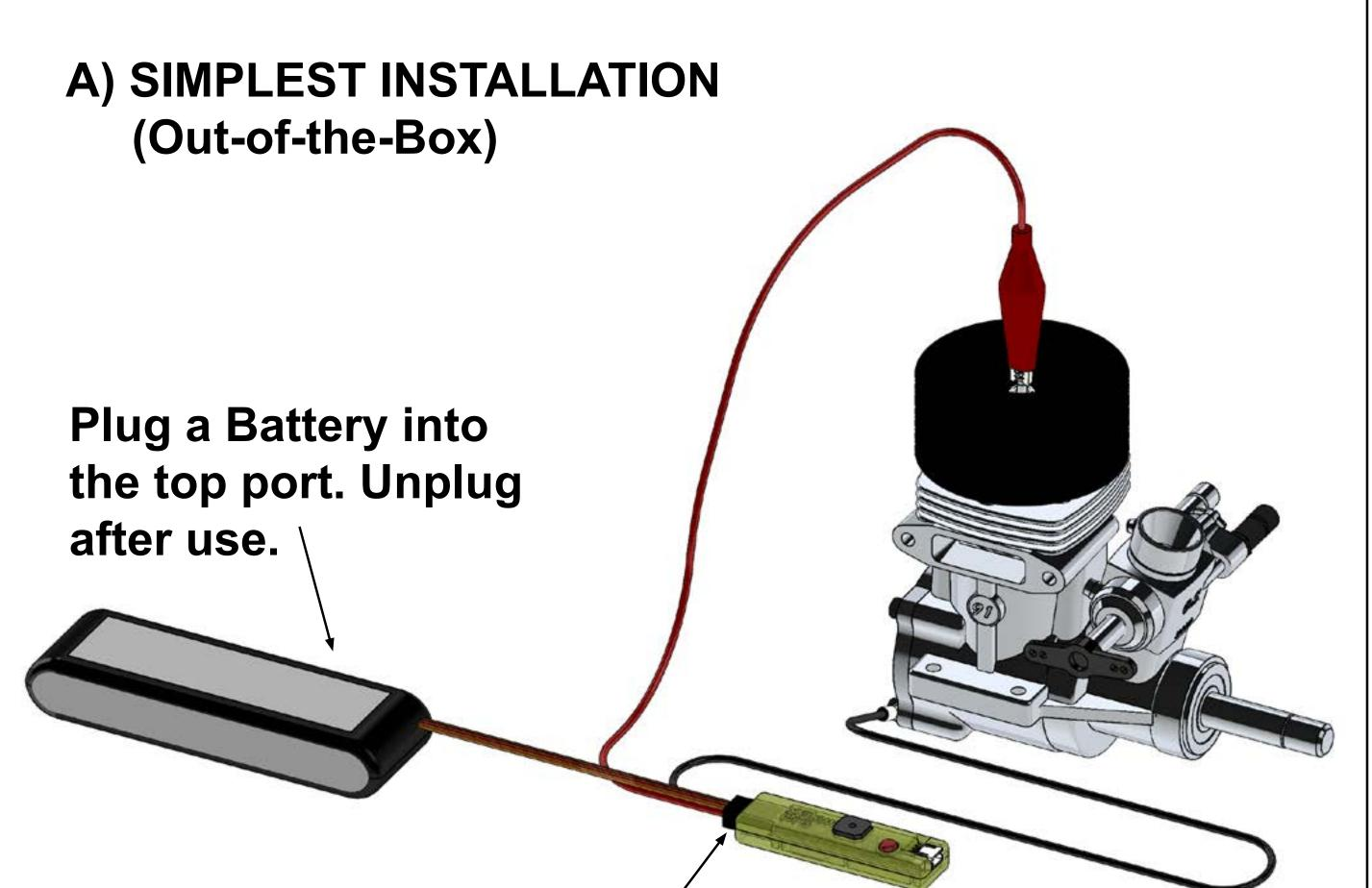
Plug the glow-plug cable into the bottom port
